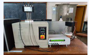
LCR Meter- High Temperature Set-up
